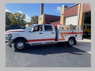
The Fire Department recently purchased a 2023 Ram 3500 Brush/Grass fire response truck. The truck is fitted with a 250-gallon water tank, 10-gallon foam cell, and CET slip-in pump.
